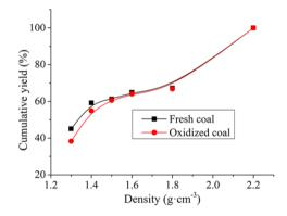
Fig. 3. Density composition of fresh coal and oxidized coal
