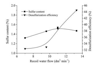
Fig. 9. Desulfurization efficiency and sulfur content of gravity concentrates at different recoil water flows
