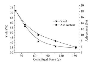
Fig. 6. Yield and ash content of clean coal of gravity concentrates at different centrifugal forces
